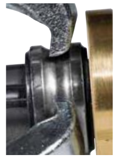
Lock on ball grooves and bearing races.
